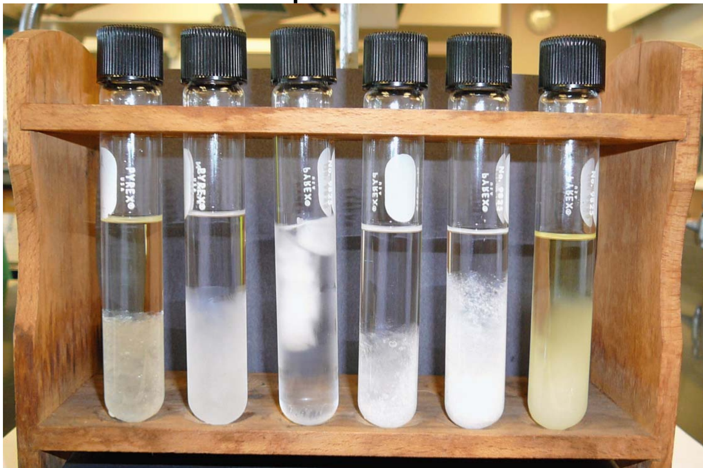
acetophenone dioxane water p -xylene acetic acid oleic acid 20°C 12°C 0°C 14°C 17°C 14°C
