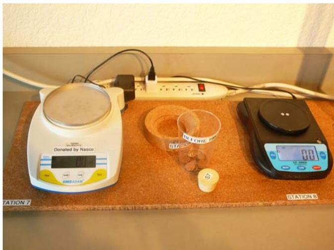
The scale on the right is the same as the scales used in Station 11. The scale on the left was donated by NASCO West and is a decigram scale. The scale on the right could have been used for both applications.
